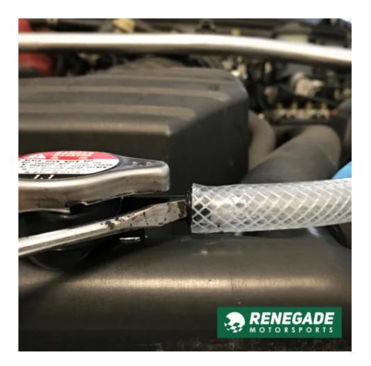
7. Install radiator cap. Pour coolant from OEM reservoir into Renegade Motorsports reservoir. Approximately 2 inches of coolant is sufficient. Enjoy!
