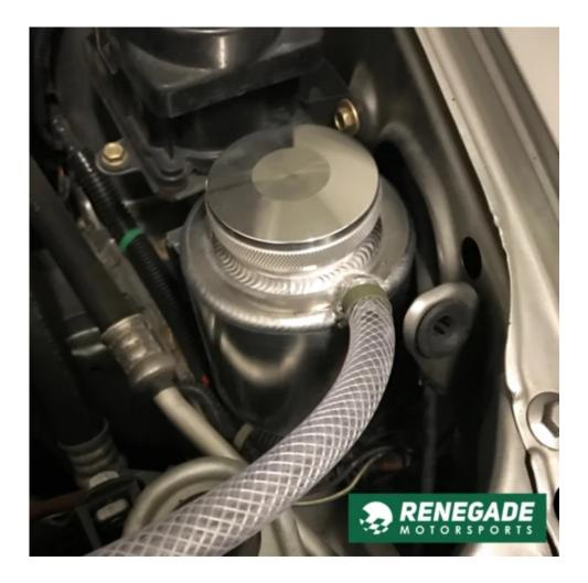
3. Slip o-ring on to radiator receptacle. (only one is used, the second is supplied as a backup).
