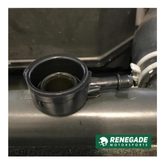
5. Use flat-head screw driver to keep o-ring in place, then slide braided PCV hose over o-ring and receptacle. Work o-ring around receptacle with screw driver to ensure o-ring has not folded or wedged unevenly. Slide spring clamp over o-ring and braided PCV hose.
